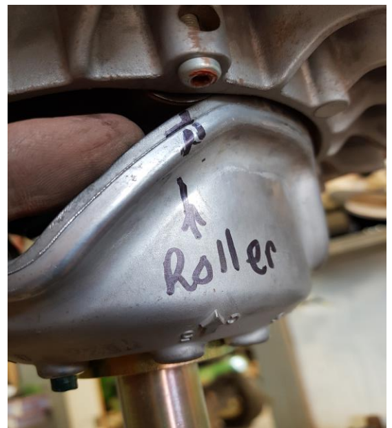
Figure #5. roller position and marks aligned (stock helix before removal shown for reference)
